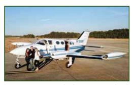
Expect to pay more for hangar space if you own a 414, particularly a 414A which has a wingspan 4.5 feet longer than the straight 414 shown here. A standard 40-foot wide T- hangar will be too small.
