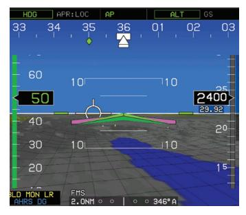
Also, when interfaced with the Genesys Aerosystems EFIS, the S-TEC 5000 can perform pitch control such as automatic step down altitude capture and hold as part of an approach.
