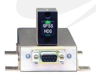
To save valuable panel space, the GPSS converter is configured as a separate panel-mounted switch and remotely-mounted control box. The control switch is  $1.32 \times .82$ ", and projects only 1" behind the panel (plus cable connector).
